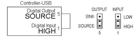
Figure 4-6: Interconnection Scheme: Simulating PNP device
