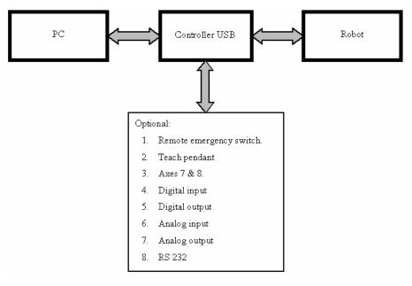
Figure 1-2: Block Diagram
