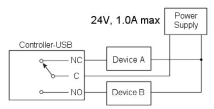
Figure 4-9: Output Relay (1 - 4) Interconnection Scheme
