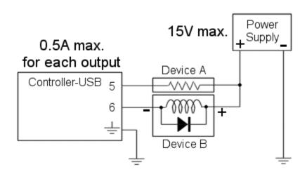
Figure 4-10: Interconnection Scheme: Sink Output
